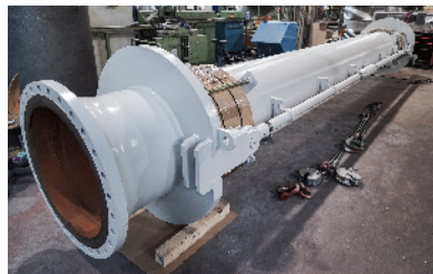
A multi-layer external epoxy coating to provide corrosion protection
