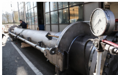
TÜV- monitored pressure test of the 7-metre long component at 28 bar
